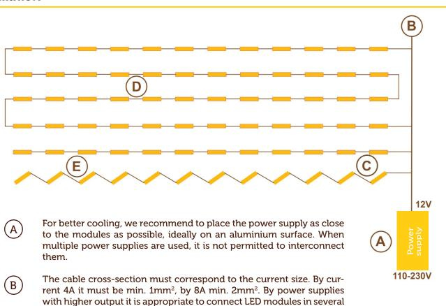
While connecting the LED modules only from one side, this line can consist of up to 20pcs of LED modules.
